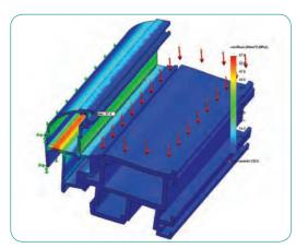
Simulation software FEM, for the calculation of the possible critical points of the system under study.
