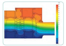
Thermal simulation software BISCO, for the calculation of the thermal transmittance value of the systems for the construction of aluminum window and door frames.
